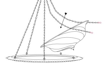
**B.** Insert the lampshade through the chains as shown in the picture.
